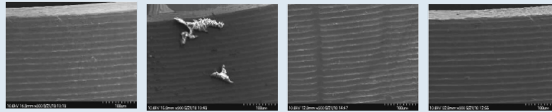
Sybron implant control photo Debris left from plastic scaler Competitor hard-ened Ti scaler No effect after PDT Ti scaler
