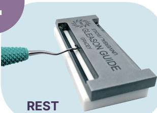
Maintain the "stop" position while dropping the terminal shank down to rest on the angled bar of the guide. This is called the "rest" position.
